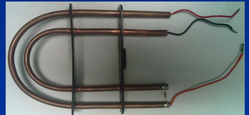
**Figure 2 - TDR Sensor Probe**
